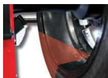
LASERLINE FOR STICK ON WEIGHT
