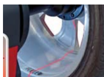
LASERLINE FOR STICK ON WEIGHT
