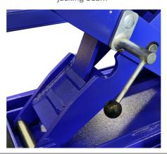
Automatically activated pneumatic safety locks & emergency cable break locks in each post
