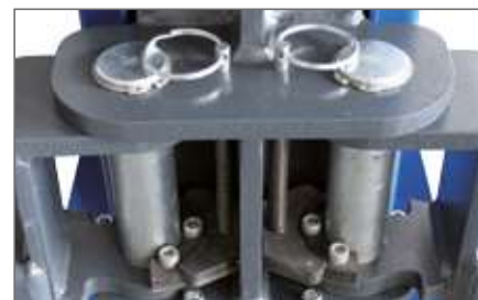
Automatic support-arm restraint with fine adjustment and manual release
